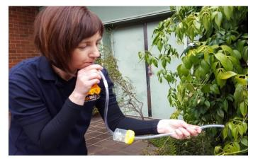
The idea is that the collector sucks on one end of the flexible tube creating suction. The insect will be sucked into the container. Because there is a filter over the end of the mouthpiece tube, the insect remains in the container.
