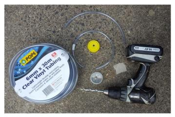
Drill a hole in the lid and the bottom of the container. Cut two pieces of plastic tubing. Mark one piece of tubing with tape – this is the mouthpiece tube for sucking. Thread this tube through the bottom of the container. Wrap the end of the mouthpiece tube with fabric and fasten with a rubber band. Screw the lid on and thread the other tube through – this is the collection tube.
