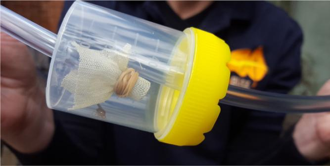
Drill a hole in the lid and the bottom of the container. Cut two pieces of plastic tubing. Mark one piece of tubing with tape – this is the mouthpiece tube for sucking. Thread this tube through the bottom of the container. Wrap the end of the mouthpiece tube with fabric and fasten with a rubber band. Screw the lid on and thread the other tube through – this is the collection tube.
